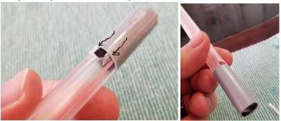
6. Measure holes according to chart (43, 50, 58, 68, 73, 83% of length from hole to end of tube)
