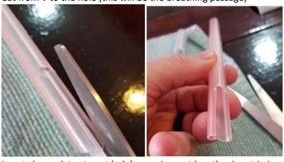
4. Insert clay cork to stop at hole's opening, cut length-wise strip in saved tubing from step 1.
